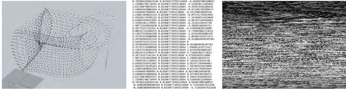
Figure 89: Point cloud encoded into matrix
